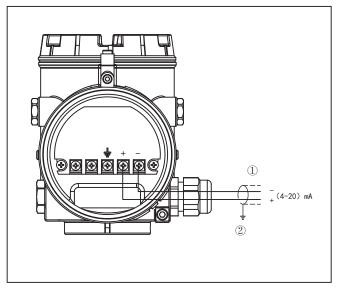
Electronics and terminal compartment, double chamber housing
